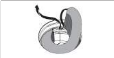
Fig. 9.6 How to remove the odour filter through the inlet opening
