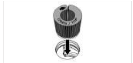
Fig. 9.8 How to insert the odour filter through the extractor opening
