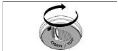
Fig. 9.9 How to place the odour filter in the end position
